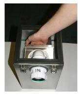
7. Slide bracket containing clean filter back under inlet pipe.
